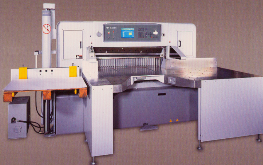
▲ CT-115E with stock lifter (fork) and bigger air table
